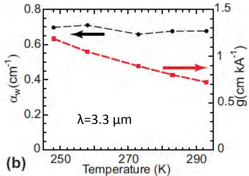
Low gain due to interface roughness
