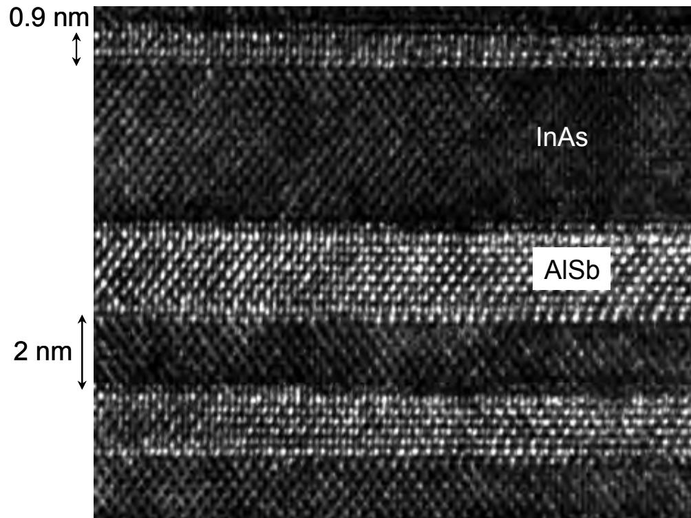
control of layer thicknesses
