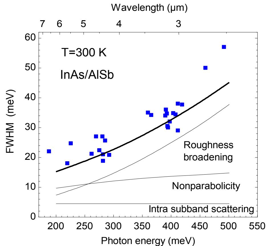
Reduction of intersubband gain :  $g \propto \frac{1}{2\gamma}$
