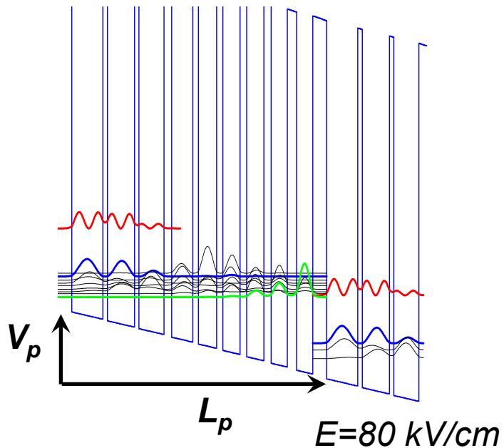
$\lambda=2.5 \mu\text{m}$  – 17 injector QWs
